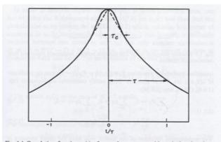
Fig. 1.4 Correlation function  $\varphi(t)$  of a random process with a single relaxation time  $\tau$ . Solid curve: real decay of the correlation function. Dashed curve: purely exponential correlation function  $\exp(-|t|/\tau)$  obtained in the Markov approximation. It deviates from the real one at small times  $|t| < \tau_c$  which in Markov approximation are microscopic times. From Lax (1960).
